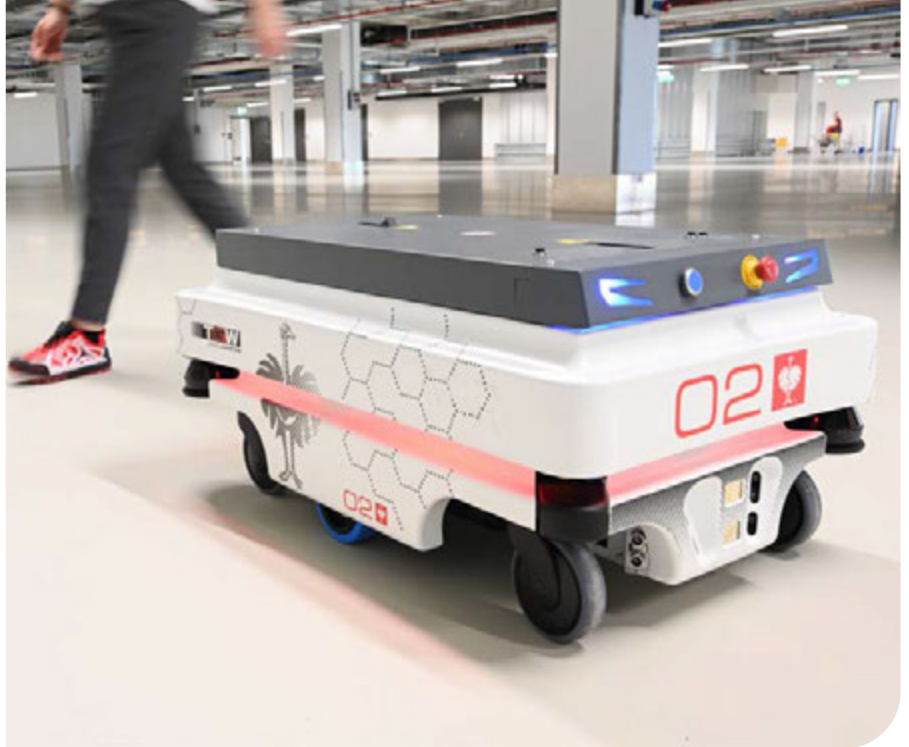
Quba. The mobile robots transport different load carriers such as pallets, cartons, and containers
